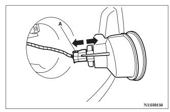
2. Push the connector (A) to disconnect and remove the light bulb.
